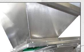
Pneumatically actuated stainless steel slide gate guillotine knife.
